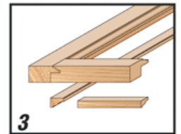
3 Assemble stiles and rails and miter cut beads to size
